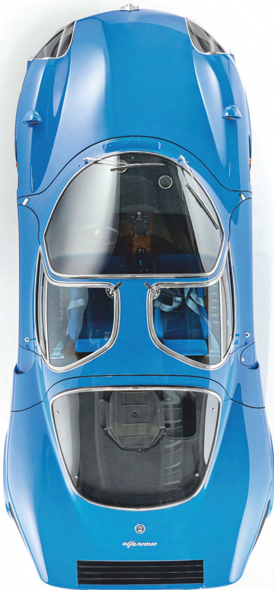
Scaglione's masterpiece is beautiful from any angle, particularly from above. Note how far the dihedral doors cut into the roof and the extra vent to cool the cabin
